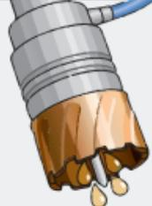
**7** Every diameter of a core drill requires a specific cutting speed (RPM) on the drilling machine. The cutting speed formula and common cutting speeds are mentioned in the footer.
