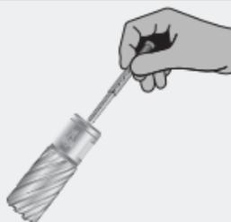
**3** The clamping screws of the tool holder must be positioned exactly on the clamping surface of the core drill. A Weldon shank core drill has two clamping surfaces, both the surfaces must be clamped.
