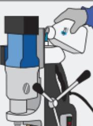
**6** Internal lubrication for the core drill is a must. Above 35 mm diameter also provide external lubrication to core drills. Only external lubrication will damage the core drills with few holes.
